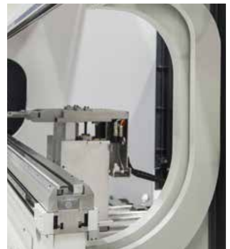
Increased table-ram/stroke/gap distance in 100 mm steps
