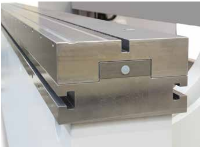
Wider table for use of multi-V dies
