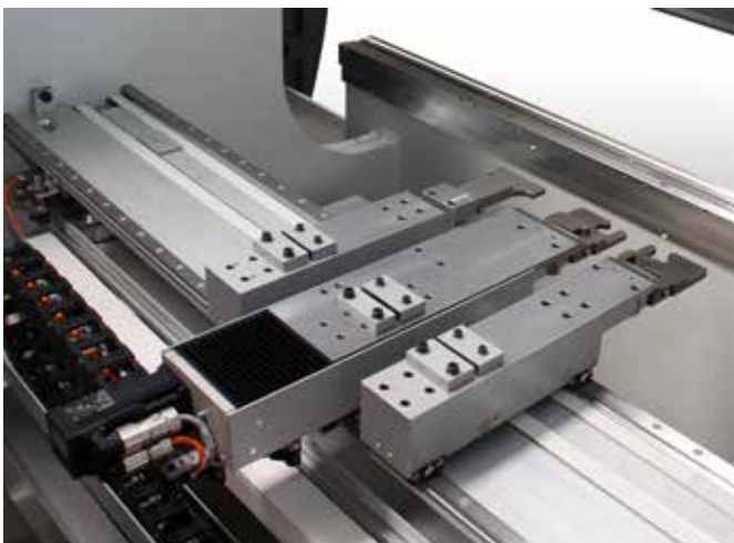
Additional backgauge finger for gauging long, small strips
